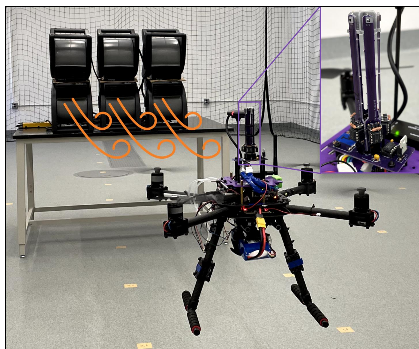
FlowDrone: A UAV with MAST (top right --- an omnidirectional flow sensor) and wind-aware control.
